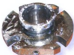
Defective mechanical seal
